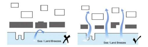
Figure 42 Waterfront buildings should avoid Wind Blockage
