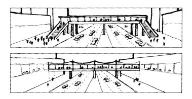
Figure 29 Linkages between Retail Malls Better than Isolated Footbridges
