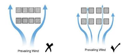
Figure 49 Gaps between Building Blocks to Enhance Air Permeability
