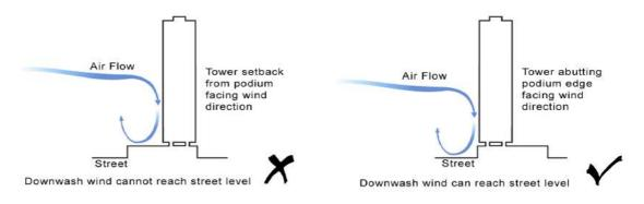
Figure 50 Towers placed to Enable Downwash Wind to Reach Street Level
