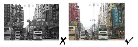
Figure 54 Projecting Signboards should be Vertical Type instead of Horizontal Type
