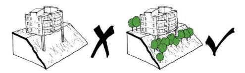
Figure 34 Minimise Negative Visual Impact of Stilted Structures
