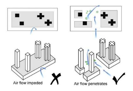
Figure 47 Reducing Site Coverage of the Podia to Allow More Open Space at Grade 11.3.3 Where appropriate, a terraced podium design should be adopted to direct downward airflow to the pedestrian level (Figure 48).
