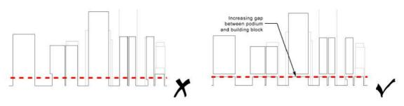
Figure 51 Gaps between the Podium and Building Blocks to Enhance Air Permeability
